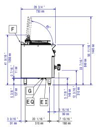
CWII = Cold Water inlet 1 (cleaning) HWI = Hot water inlet D = Drain
